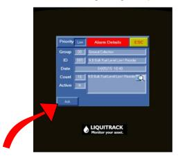
The alarm history will remain in memory for upto 12 records. these records can also be viewed by proceeding to the [Alerts] icon on the main menu. The records can then be scrolled through by using the on screen arrows.
