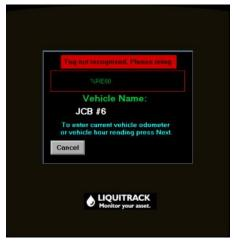
Tag not recognised. This indicates the ibutton is not programmed on the system or the tag reading process experienced a problem. To re-tag, please wait 5 seconds.
